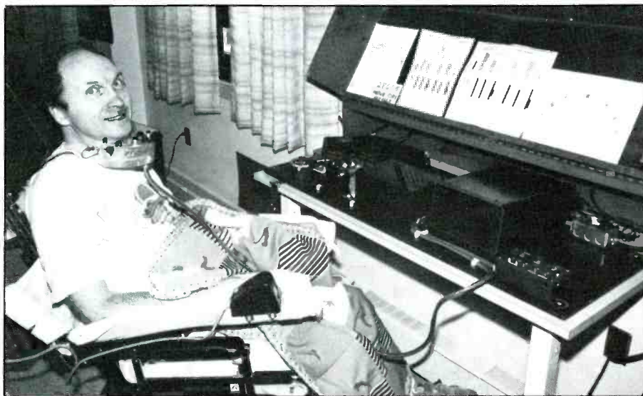
Although paralyzed from the neck down, Rob Michon, WD80TI, of Ann Arbor, Michigan, uses a specially made "neck console" to operate his transceiver. Rob is a member of Handi-Hams and is working on upgrading from Advanced to Extra Class. His custom-engineered control system was designed and built by Roger Place, W8ZRF, of Ypsilanti, Michigan.
