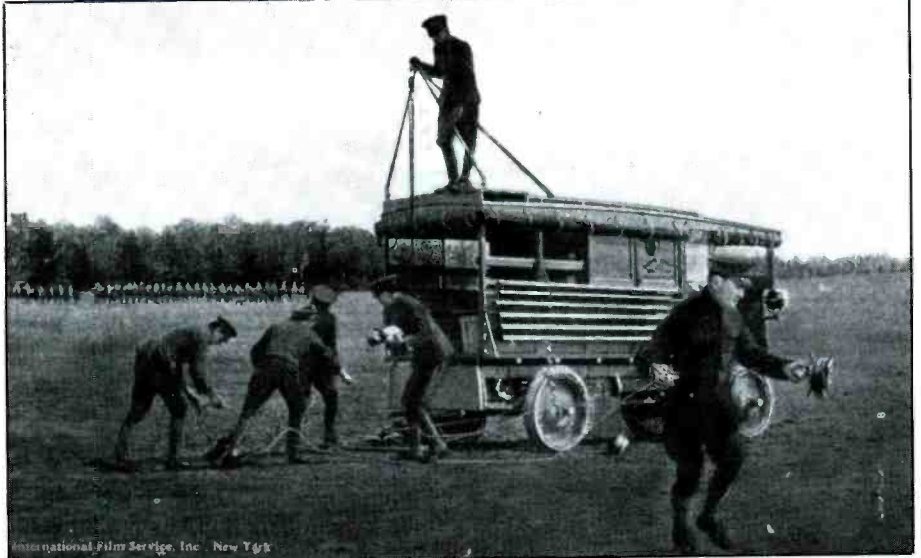
A WWI U.S. Army wireless truck required a crew of six to string out endless yards of low frequency antenna and counterpoise wires. The tripod on the roof was needed to put up the masting. Six mast sections are shown mounted on the side of the truck. Solid hard-rubber tires were used because they were standard equipment and also puncture proof, even though they had a low comfort rating. Pneumatic tires had already been around for more than 20 years but were still an optional extra. They didn't become standard equipment until 1924.
