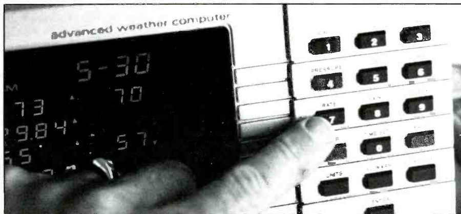
The "rate" key lets you see what is changing over the last few hours. (Photo courtesy Gordon West).
