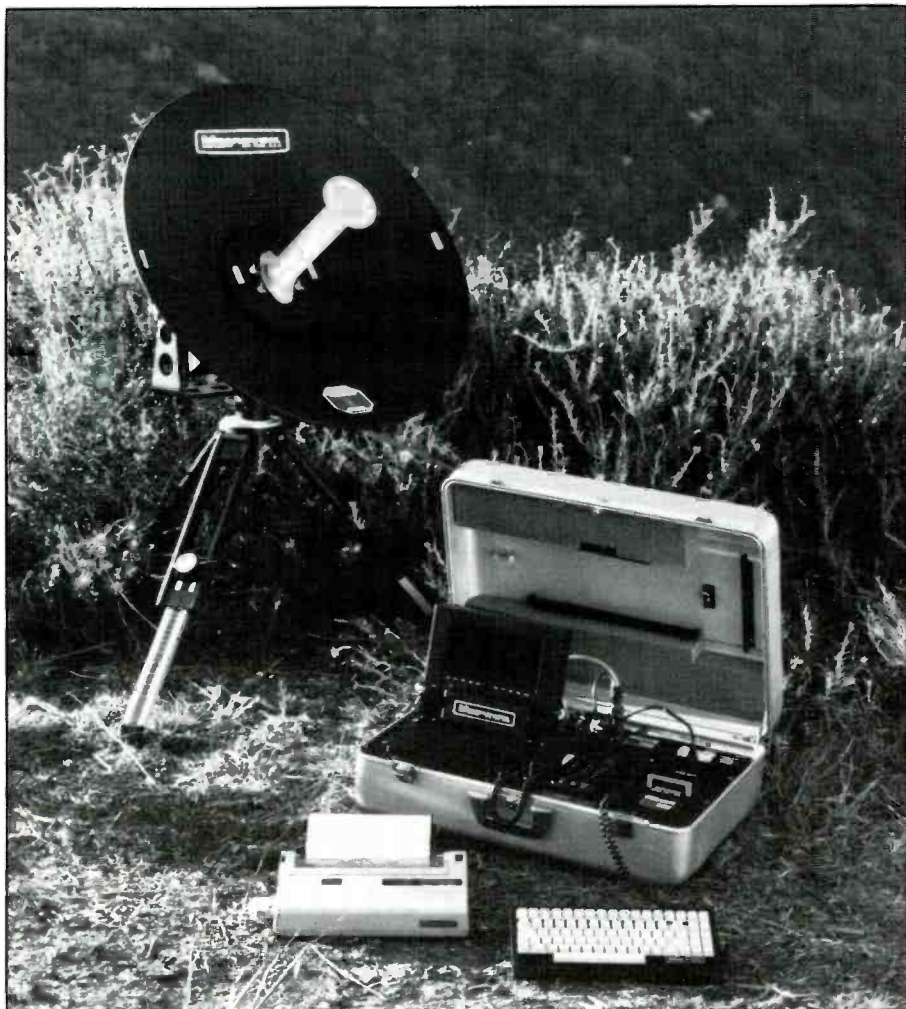
The Magnavox MX-2400T; transportable satellite comms in a suitcase
