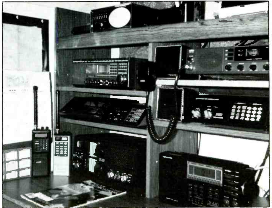
Here's the well-equipped listening post of John H. Lingaton of Duke Center, Pennsylvania. His scanners include the following: Bearcat III, Bearcat 210XLT, Regency MX3000, Realistic Pro-2020, Bearcat 200XLT and Realistic Pro-38. John has been a radio buff for 35 years.
